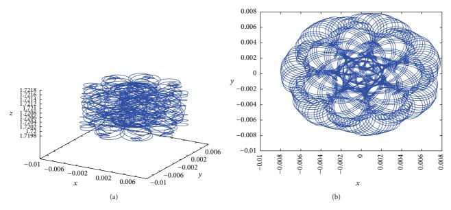
FIGURE 1: Trajectory calculated with MPE method supplied with the Verlet algorithm.
