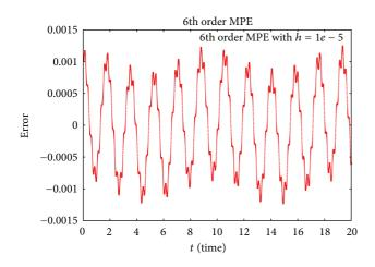
FIGURE 4: Errors of the numerical scheme: 6th order extrapolation scheme with Verlet method as kernel ( $h = 10^{-5}$ ).
