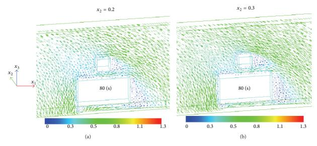
FIGURE 10: Velocity vectors around 3D AGV model.
