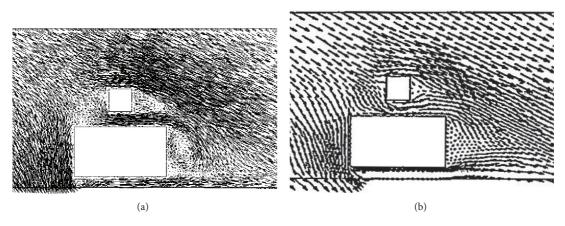
FIGURE 8: Velocity vectors around the AGV (a) current 3D results; (b) Kanayama et al.'s 2D results.
