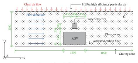
FIGURE 1: A moving AGV in a cleanroom.
