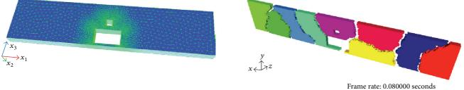
FIGURE 6: The meshing of the 3D AGV model.
