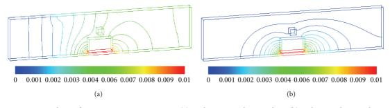
FIGURE 12: Isolines of contaminants concentration. (a) Without vertical external air; (b) with vertical external air.
