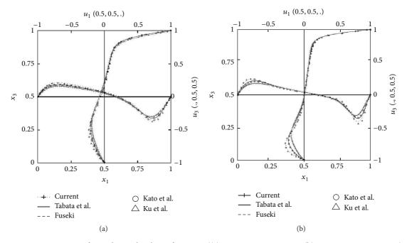
FIGURE 4: Comparison of  $u_1$  and  $u_3$  at the plane of  $x_2 = 0.5$ . ((a):  $50 \times 50 \times 50$ , Re = 400; (b):  $80 \times 80 \times 80$ , Re = 1,000).
