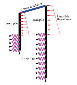
FIGURE 5: The conceptual calculation model for portal double-row stabilizing pile.
