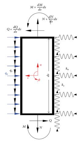
FIGURE 2: The free-body diagram of infinitesimal isolated segment of pile.
