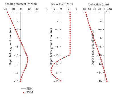
FIGURE 6: Comparison of internal force and deflection of front row pile between the boundary value method and FEM.
