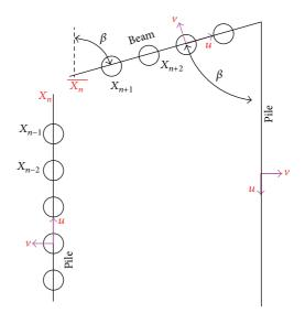
FIGURE 3: Scheme of local coordinate system transformation between pile and connection beam.
