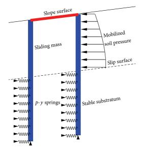
FIGURE 1: The uncoupled analysis model for the double-row portal stabilizing piles.
