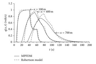
FIGURE 3: Departing flow distribution at upstream intersection.
