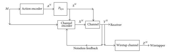
FIGURE 6: Wiretap channel with action-dependent channel state information and noiseless feedback.
