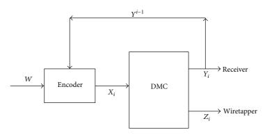
FIGURE 3: The general wiretap channel with noiseless feedback.
