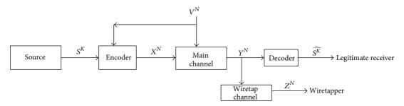
FIGURE 5: Wiretap channel with noncausal channel state information.
