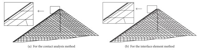
FIGURE 6: Two-dimensional finite element mesh.
