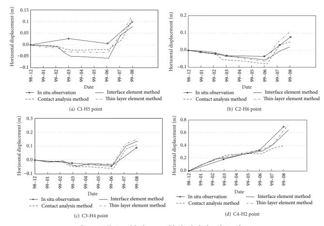
FIGURE 10: Horizontal displacement of the dam body along the interface.
