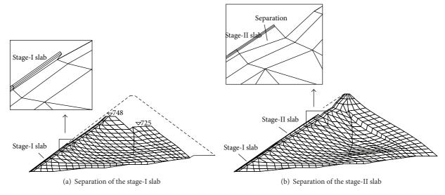
FIGURE 11: Separation of the slab from the cushion layer at different stages (interface element method).
