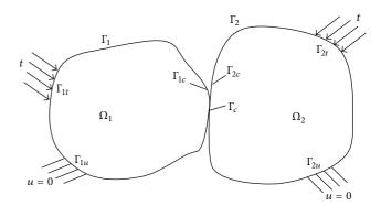
FIGURE 1: Contact of two deformable bodies.
