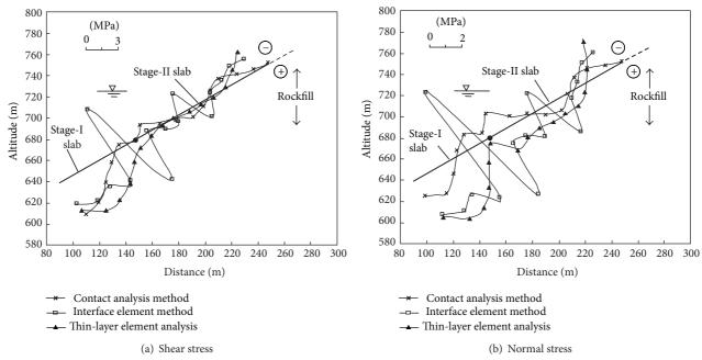
FIGURE 14: Comparison of stresses in the concrete face slab at completion of the dam body construction.
