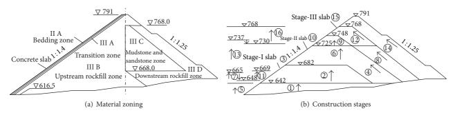
FIGURE 5: Material zones and construction stages of Tianshengqiao-I CFRD.
