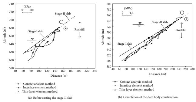
FIGURE 13: Comparison of normal contact stress along the interface.
