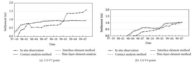
FIGURE 9: Settlement of the dam body along the interface.
