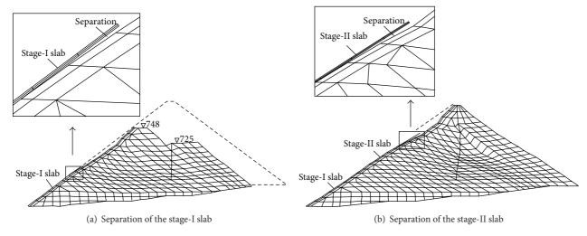
FIGURE 12: Separation of the slab from the cushion layer at different stages (contact analysis method).
