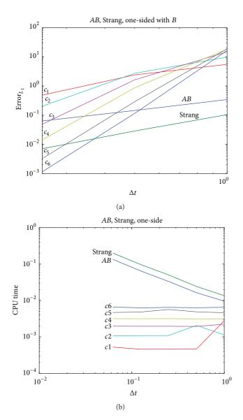
FIGURE 5: Numerical errors and CPU time of the standard splitting scheme and the iterative schemes with Zassenhaus formula, where we have at least 1,..., 4 iterative steps.
