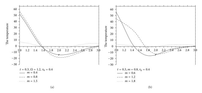
FIGURE 3: Variation of temperature  $\theta$  with radius *r* (thermoelastic diffusion nonhomogeneity medium).
