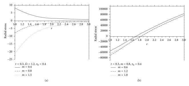
FIGURE 5: Variation of radial stress  $\sigma_{rr}$  with radius r (thermoelastic diffusion nonhomogeneity medium).
