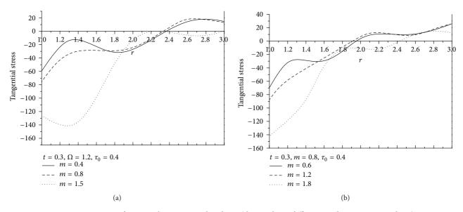
FIGURE 6: Variation of tangential stress  $\sigma_{\phi\phi}$  with radius r (thermoelastic diffusion nonhomogeneity medium).
