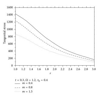
FIGURE 10: Variation of tangential stress  $\sigma_{\phi\phi}$  with radius r (thermoelastic nonhomogeneity medium).
