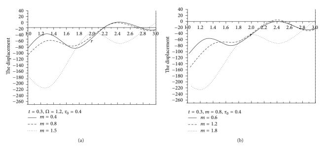
FIGURE 4: Variation of displacement *u* with radius *r* (thermoelastic diffusion nonhomogeneity medium).
