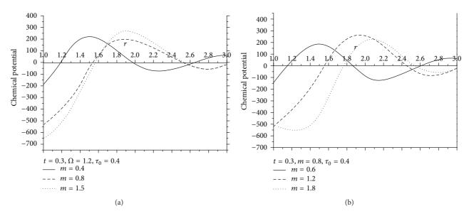
FIGURE 1: Variation of chemical potential P with radius r (thermoelastic diffusion nonhomogeneity medium).
