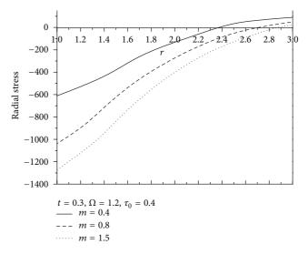
FIGURE 9: Variation of radial stress  $\sigma_{rr}$  with radius r (thermoelastic nonhomogeneity medium).
