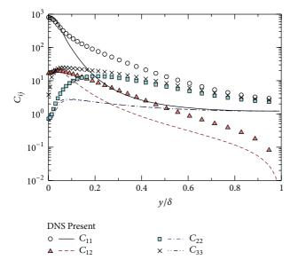
FIGURE 12: Mean conformation tensor for  $\text{Re}_{\tau}$  = 395,  $\text{Wi}_{\tau}$  = 30, and  $\beta$  = 0.5.
