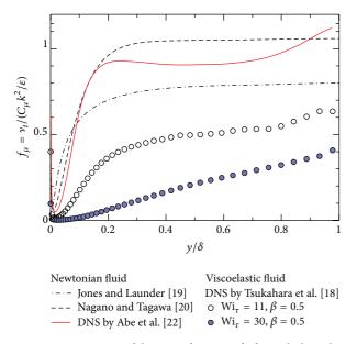
FIGURE 1: Comparison of damping function  $f_{\mu}$  for turbulent channel flow at Re<sub>r</sub> = 395.
