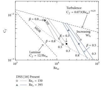
FIGURE 7: Frictional coefficient.
