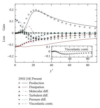
FIGURE 13: Budget of turbulent kinetic energy for drag-reducing viscoelastic fluid in turbulent channel flow at  $\text{Re}_{\tau} = 395$ ,  $\text{Wi}_{\tau} = 30$ , and  $\beta = 0.5$ .
