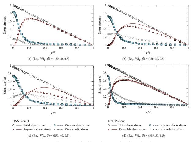
FIGURE 11: Shear stress profiles of drag-reducing viscoelastic flow in channel.
