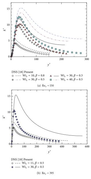
FIGURE 9: Same with Figure 6, but with respect to turbulent kinetic energy,  $k^+$ .
