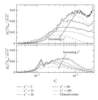
FIGURE 3: Premultiplied one-dimensional spanwise energy spectra of streamwise velocity fluctuation in drag-reducing viscoelastic flow at Re<sub>r</sub> = 395. (a) Wi<sub>r</sub> = 10,  $\beta$  = 0.8 and (b) Wi<sub>r</sub> = 30,  $\beta$  = 0.5.
