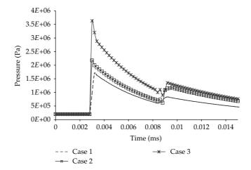
Figure 6: Pressure evolution as function of time with hydrogen mass fraction cases.
