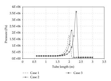
**Figure 4:** Pressure evolution along shock tube and as function of hydrogen mass fraction in air (case 1: 1.5%, case 2: 2.5%, case 3: 5%).
