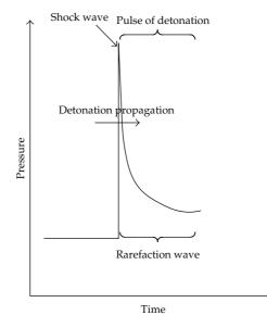
Figure 2: Structure of the pulse detonation.
