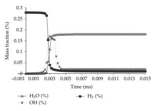
**Figure 9:** Mass fraction profile of the  $H_2$ ,  $OH^-$  and products  $H_2O$ .
