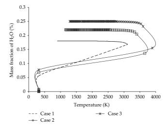
Figure 8: Mass fraction as function of temperature for each hydrogen concentration in air.
