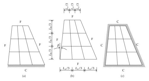
**Figure 5:** The 3 meshes adopted for the 10 mm aluminum trapezoidal plates with 1 mm PZT-5H layers perfectly bonded on both the upper and lower surfaces having various boundary conditions (the number of Fourier terms: p = q = 5,  $L_a = 0.1$  m).
