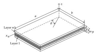
Figure 1: The configuration of a laminated composite plate.
