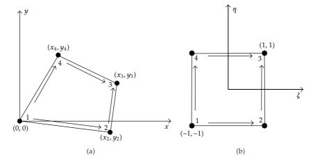
Figure 2: The coordinate transformation of a quadrilateral element.
