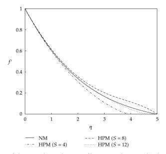
**Figure 2:** Comparison of dimensionless velocity profiles versus the normalized coordinates using the Keller's box numerical method with the results obtained by HPM at Ec = 0.1, m = 0, Pr = 6.2,  $\varphi = 0.2$ , and Mn = 0.2.
