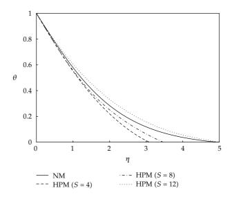
**Figure 7:** Comparison of dimensionless temperature profiles versus the normalized coordinates using the Keller's box numerical method with the results obtained by HPM at Ec = 0, m = 0, Pr = 6.2,  $\varphi = 0.2$ , and Mn = 0.2.
