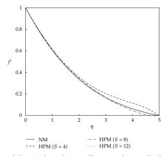
**Figure 6:** Comparison of dimensionless velocity profiles versus the normalized coordinates using the Keller's box numerical method with the results obtained by HPM at Ec = 0, m = 0, Pr = 6.2,  $\varphi = 0.2$ , and Mn = 0.2.
