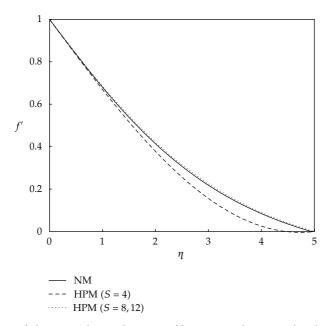
**Figure 4:** Comparison of dimensionless velocity profiles versus the normalized coordinates using the Keller's box numerical method with the results obtained by HPM at Ec = 0.1, m = 0, Pr = 6.2,  $\varphi = 0.2$ , and Mn = 0.
