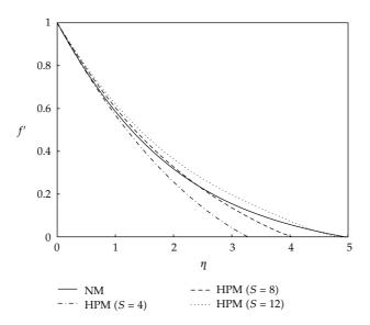
**Figure 8:** Comparison of dimensionless velocity profiles versus the normalized coordinates using the Keller's box numerical method with the results obtained by HPM at Ec = 0.1, m = 0.1, Pr = 6.2,  $\varphi = 0.2$ , and Mn = 0.2.
