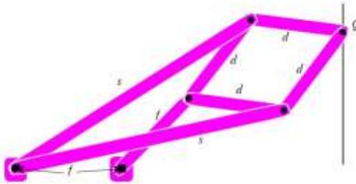
Figure 16.8 Linkage for drawing a straight line
