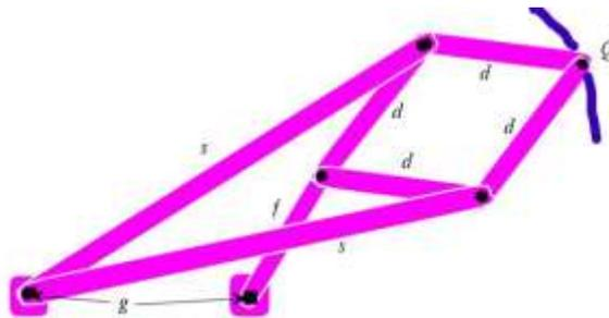
Figure 16.9 Peaucellier-Lipkin linkage modified to draw the arc of a circle
