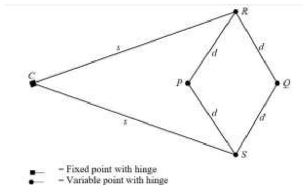
Figure 16.7 A linkage for constructing an inversion
