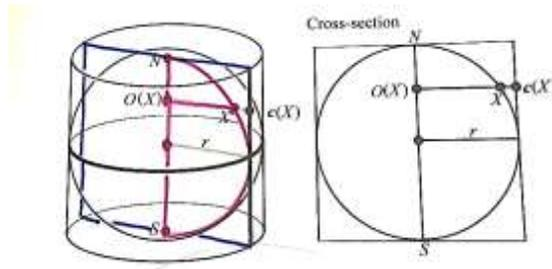
Figure 14.2 Cylindrical projection
