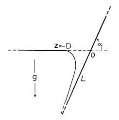
supported by a semi-infinite horizontal plane, and is bounded on the right by an infinite plane inclined at an angle  $\alpha$  with the horizontal. The flow is downward through an open slot in the horizontal plane into a jet with a free boundary extending to infinity. This family includes the case of the symmetric jet from a slot, obtained when  $\alpha = \pi/2$  by reflecting the flow across the vertical boundary.
