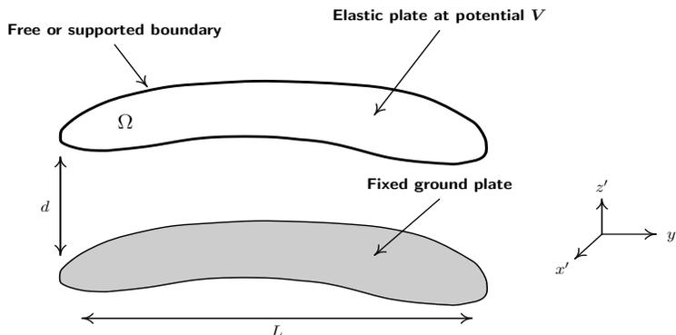
FIG. 1. Schematic plot of the MEMS capacitor with a deformable elastic upper surface that deflects towards the fixed lower surface under an applied voltage
