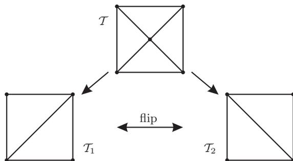
**FIGURE 5.** Nonuniqueness of irreducible triangulations. In the lower part is shown a flip, while the two moves above are edge-contractions leading to two different irreducible triangulations from  $\mathcal{T}$ .
