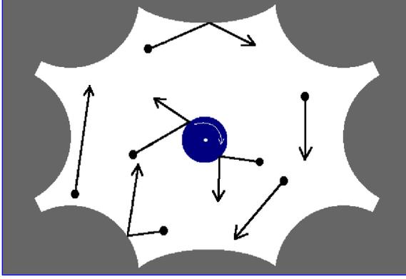
FIG. 2. Example of a mechanical system that motivated the present study: Particles in a domain  $\Gamma$  (white) are scattered as they are reflected off  $\partial\Gamma$ , and energy is exchanged when a particle collides with the rotating disk (blue) nailed down at the center of the domain.
