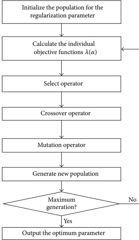
FIGURE 1: Flow chart for the calculation of regularization parameter based on GA.
