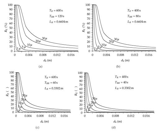
**Figure 5:** Prediction of the inclusion removal rate in a continuous casting tundish, (a) Constant  $T_R$  and  $L_B$ , (b) Decrease of  $T_R$  in 200 s, (c) Decrease of  $L_B$  by half, and (d) Decrease of  $T_R$  and decrease of  $T_R$  and decrease of  $T_R$  and  $T_R$  and T
