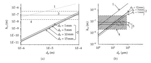
**Figure 1:** The critical film thickness ( $h_{cr}$ ) calculated as a function of the inclusion diameter ( $d_p$ ), (a) alumina inclusion and (b) silica inclusion [13].
