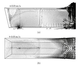
**Figure 7:** Velocity profiles inside the tundish without argon injection, (a) At the symmetric-longitudinal plane and (b) At the tundish steel level.
