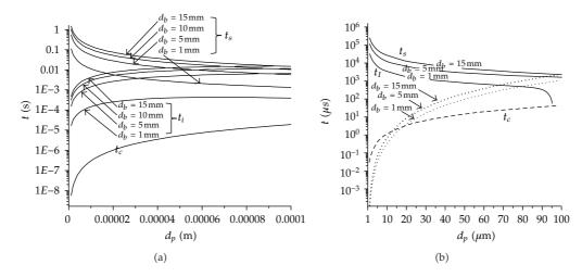
**Figure 2:** Relationship of the Inclusion Diameter to the collision, sliding and induction times. (a)  $t_i$  calculated using the Nguyen's equation and (b)  $t_i$  reported by Zhang and Taniguchi [13].
