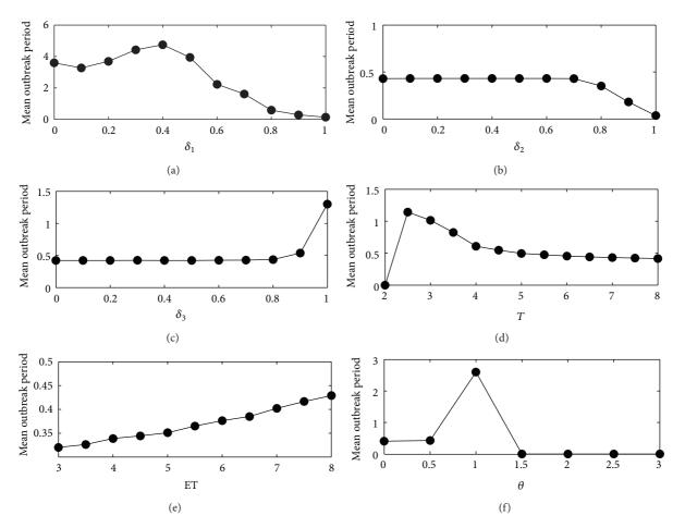
FIGURE 9: The relationship between mean outbreak period and the parameters  $\delta_1$ ,  $\delta_2$ ,  $\delta_3$ , *T*, ET, and  $\theta$  of model (11). The other parameters are the same as Figure 8.
