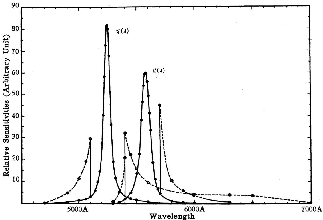
Fig. 3.1 Relative Sensitivities of the Photometer using the GreenLine or the Control Filter,  $\rho_1(\lambda)$ ,  $\rho_2(\lambda)$  in Arbitrary Unit.
