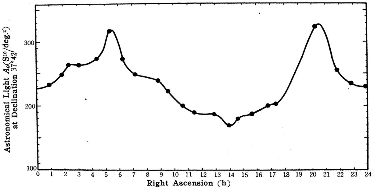
Fig. 6.1 Mean Astronomical Light in  $5250 \text{ \AA}$  against Right Ascension at the Constant Declination  $37^{\circ}42'$ .
