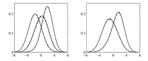
Figure 4: Approximation error for distributions of observations given boundary (left) and initial states (right): 3 summands, 3 integration points (dotted), 4 summands, 5 integration points (dashed), true (solid)
