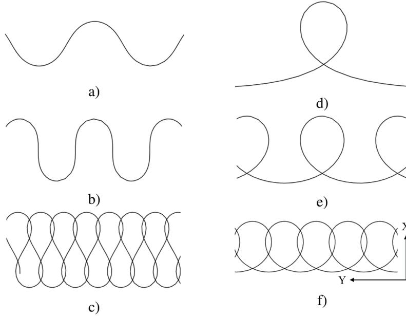
**Figure 7.** Types of Elastica: a) shows type Ia, b) is the rectangular elastica ( $a = 0$ ), c) is type Ib, and d)-f) correspond to type II.
