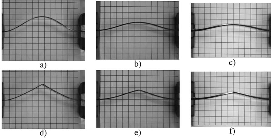
**Figure 2.** Press experiments of elastic beam: a) - c) are elastic panels with critical curvature whereas d) - f) are of  $\Lambda_{\phi_0}$  shapes of elastic panels which appear at the bounce-back of the separated pieces of panels and they behave like separated pieces of panels and they behave like continuum beams. The thickness  $\delta$  of a) and d) are 2.0[mm], b) and e) correspond to 3.0[mm] and c) and f) to 5.0[mm].
