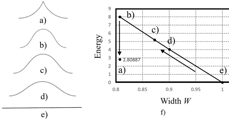
**Figure 8.** A transition: a) - e) shows the orbit from elastica to  $\Lambda_{\phi_0}$  elastica from e) to a), whereas for the orbit, the total energy is illustrated in f). The width of b) is the same as that of a), which corresponds to the critical width. In the computation, we let  $L = 1$  and  $\kappa = 1$ .
