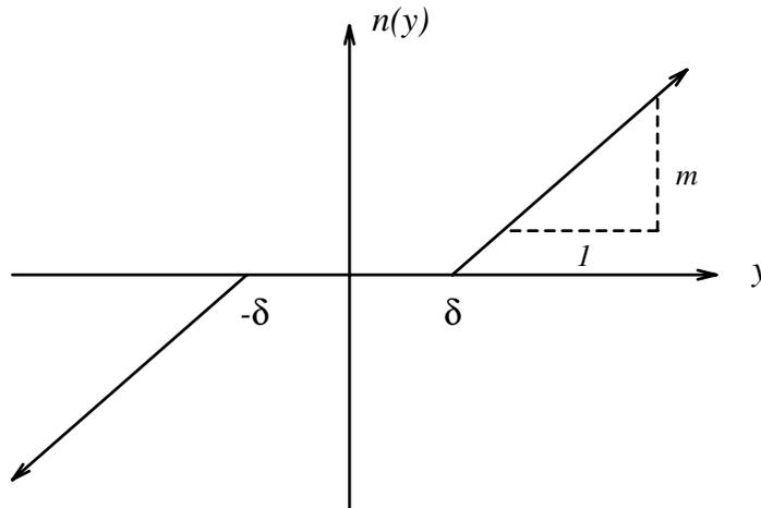
FIGURE 2. Threshold nonlinearity.
