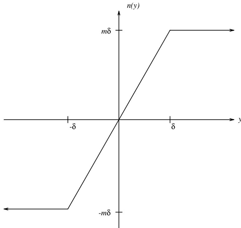
FIGURE 3. Saturation function:
