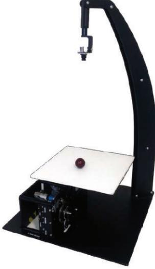
FIGURE 1: 2D Ball Balancer.
